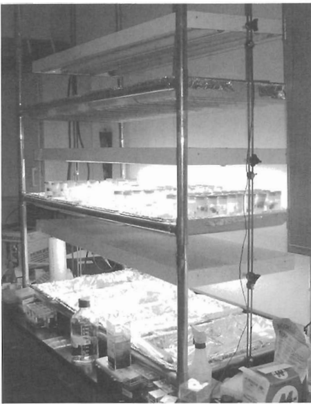
Figure 3: My light stand for tissue cultures. Only two shelves are in use in the picture. The stand is about 2 m high by 1.7 m wide by 0.7 m deep (6 ft by 5 ft by 2 ft).
