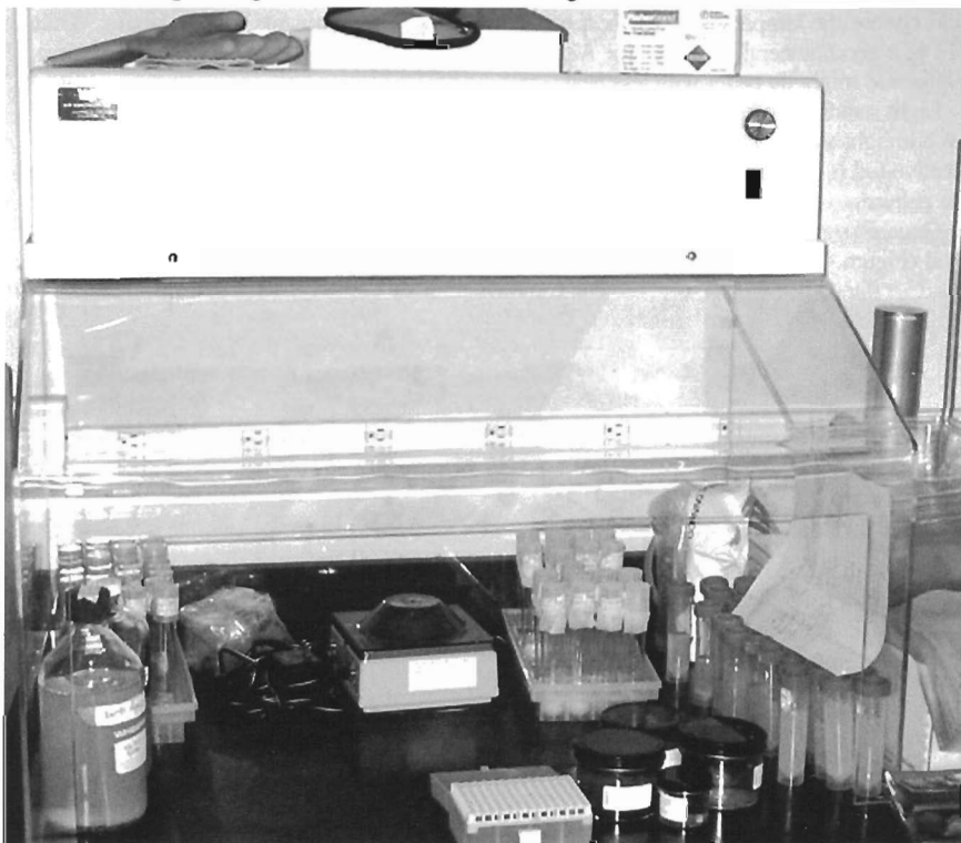
Figure 2: A laminar flow hood in my lab. This model cost about US$1500 (in 2003) and is about 1.3 m wide by 0.8 m deep by 1 m high (4 ft by 2.5 ft by 3 ft).
